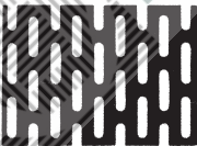
No. 53 \frac{1}{8} " x \frac{1}{2} " slot \frac{1}{2} " bar. Side staggered. 38% open area.
